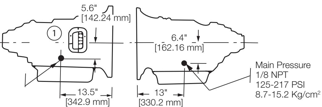
**NOTE:** Use cooler return port for PTO lubrication. The T fitting is to be installed in the port that is coming from the cooler back to the transmission.
