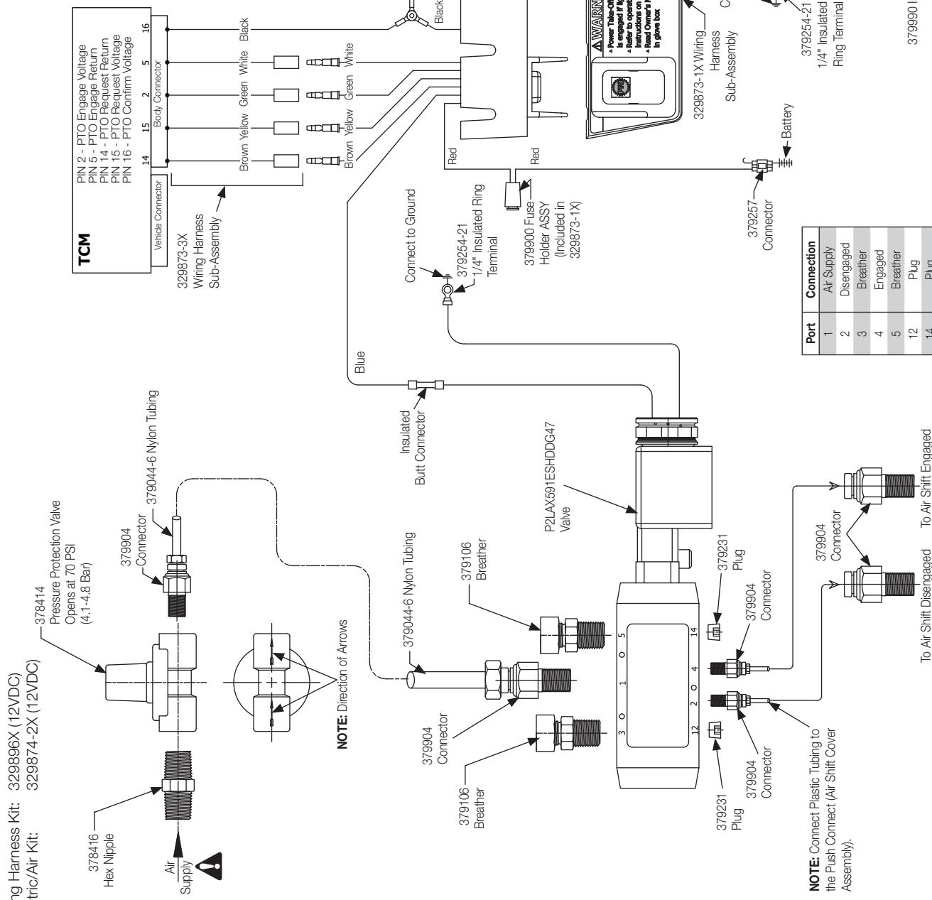
**⚠️ WARNING:** Connect directly to the air supply. Do not use tubing between the air supply and the pressure protection valve.
