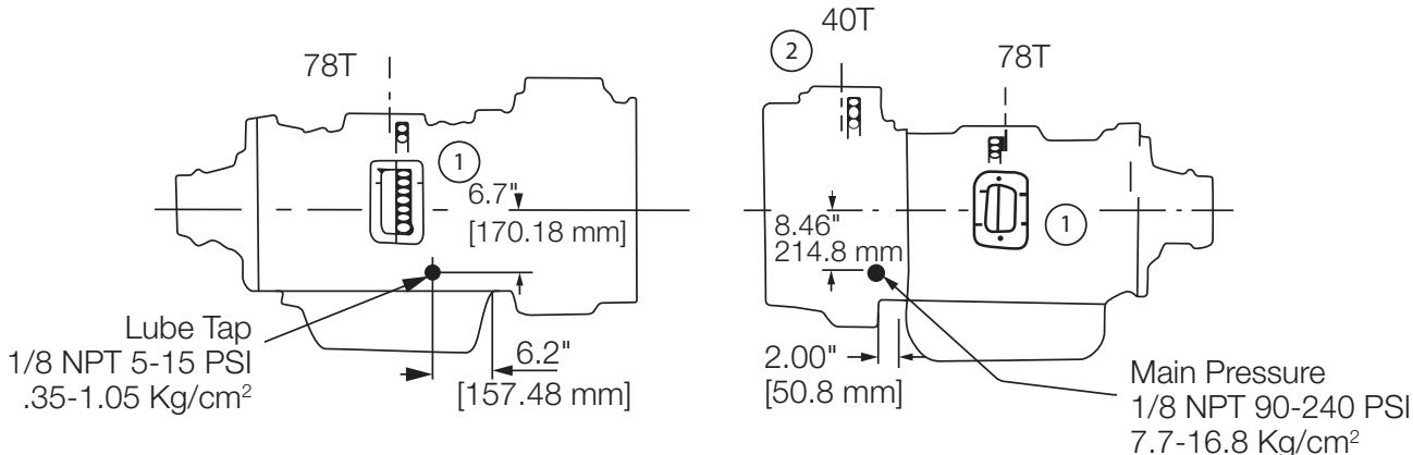
1. Converter driven PTO Drive Gear.
