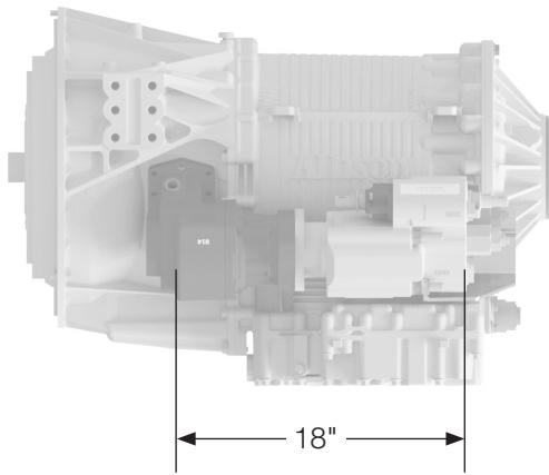
To ensure proper bracketing, brackets must attach at two or more transmission bolt locations as well as two or more pump (bolt) locations. Please reach out to your transmission manufacturer for proper bracket mounting locations.
