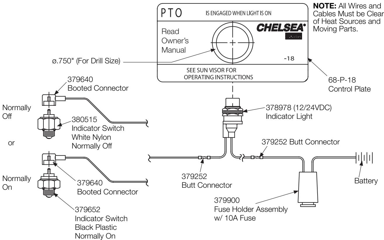
**CAUTION:** Indicator switches are capable of 0.5A maximum.
