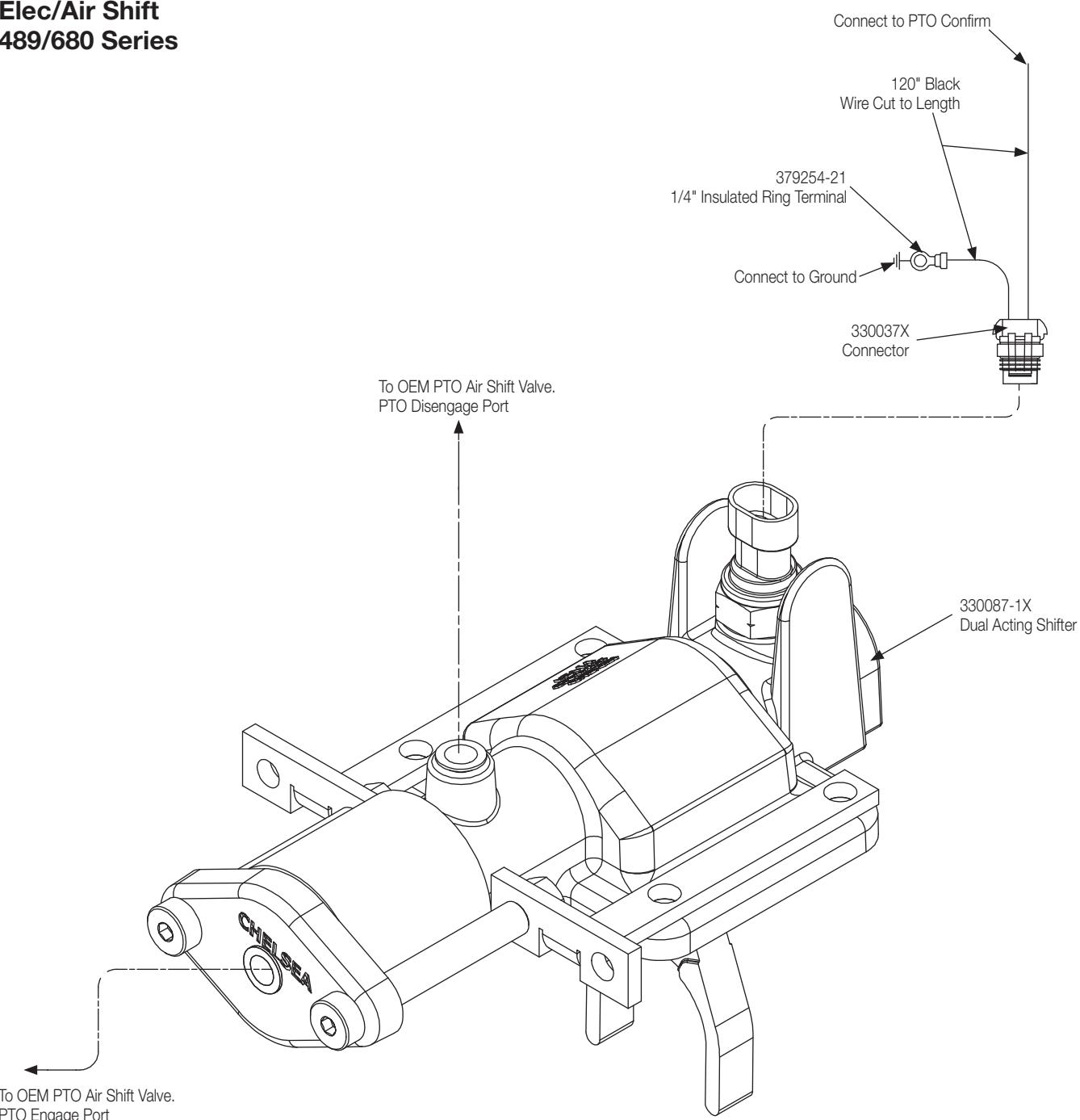
**NOTE:** If a 12VDC Elec/Air Pneumatic Valve kit is needed, Order 329874-2X
